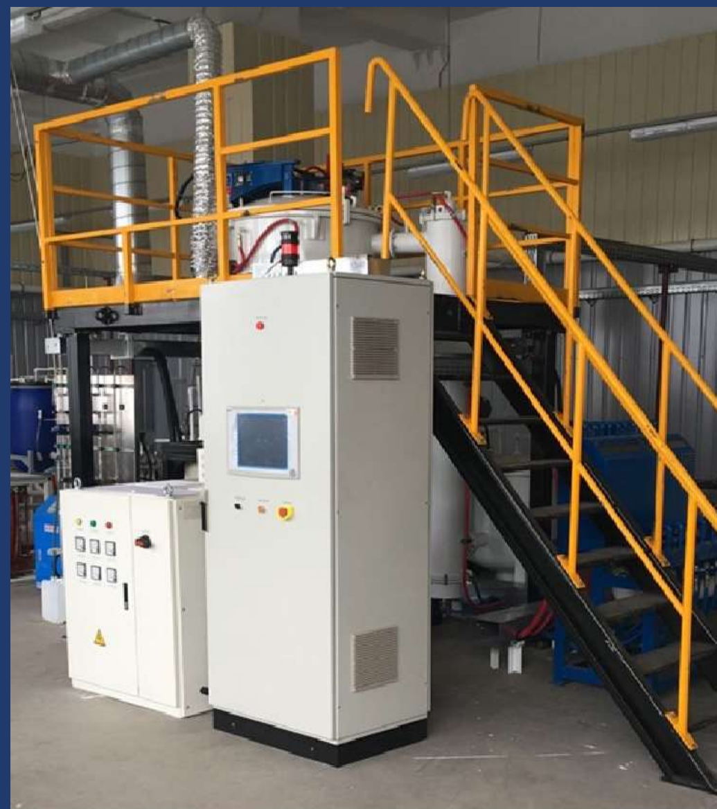
Silicon carbide Deposition Plant (MTS)
