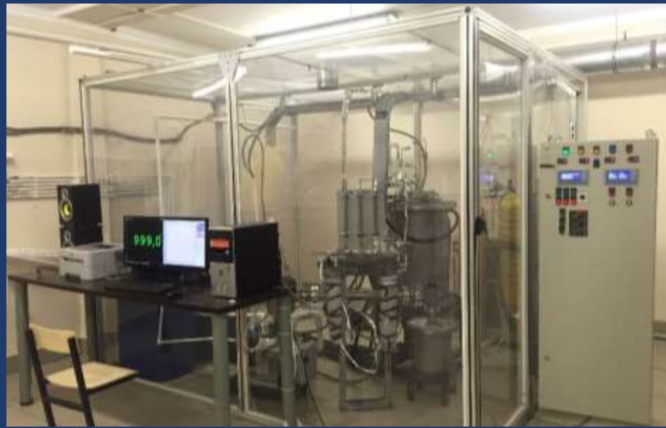
Pyrolytic Boron Nitride Deposition Plant 1.0
